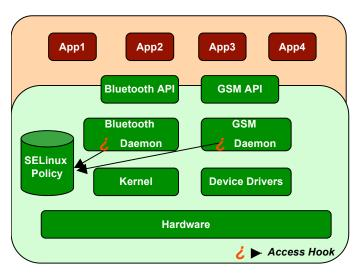
The mobile phone has various critical resources that should not be misused. The aim is to mediate access by untrusted applications to these resources. Access hooks are inserted into active processes that interact with the resources. Every time an application requests access to a resource, the permission is granted or denied depending on a policy look-up.
