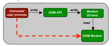
An untrusted process should not be allowed to write to a trusted object because this can interfere with phone critical applications like the interface for the GSM daemon. We do the following:
